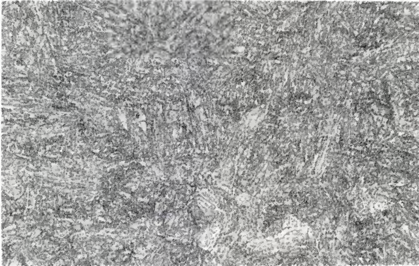
5(b) Mid-wall - Martensite - Bainite
